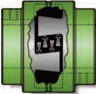
**Load-Lock Design...** is simple and effective. The drive lug configuration is tapered from top to base, as are the mating lugs of the opposing coupling hub. Under load, the insert conforms to the tapers, inter-locking the two hubs. This load-lock design protects bearings and equipment by eliminating end thrust in both directions.... and it requires only one set-screw in each hub.
